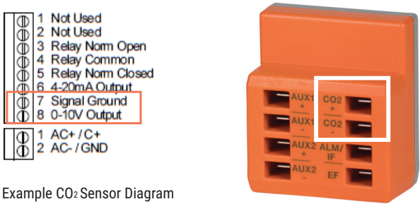
Example CO 2 Sensor Diagram
